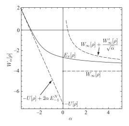
FIG. 2. The functional  $W_{\alpha}[\rho]$  (in Hartree atomic units) as a function of the dimensionless coupling strength parameter  $\alpha$  (solid curve), as modeled in Sec. III, using the five functionals  $E_x[\rho]$ ,  $U[\rho]$ ,  $W_{\infty}[\rho]$ ,  $W_{\infty}'[\rho]$ , and  $E_{-1}^N$  for the Be atom (see Table I).
