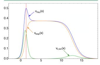
Figure 11. Hartree-XC potential,  $v_{Hxc}(x)$ , and its contributions  $v_{c,\text{kin}}(x)$  and  $v_{\text{resp}}(x)$ , for a=2, b=1, and R=8. The red dashed line highlights the position where  $x = a_R$ .
